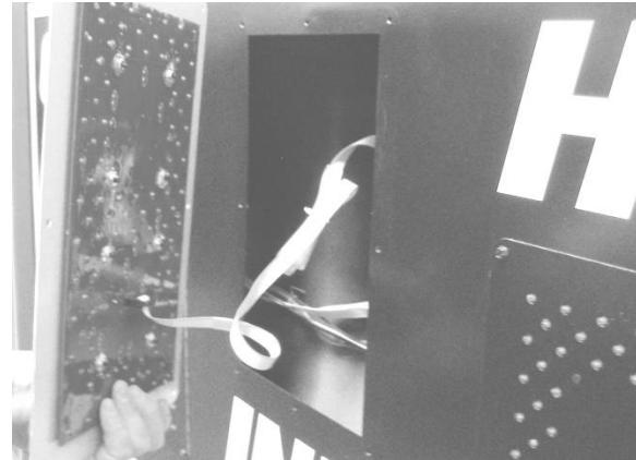
If your purpose in removing the LED assembly was to provide access to the components behind it, you may skip the next part about removing and replacing the LED printed circuit board.
